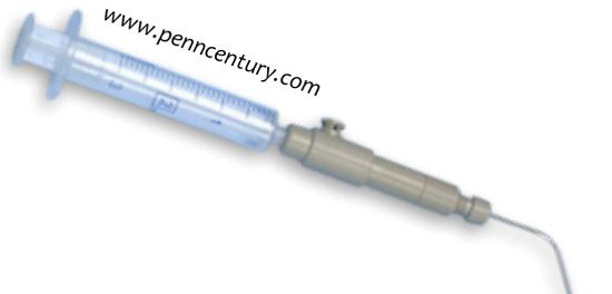
\* Dry nebulisation of VA onto the triple cell co-culture at the air-liquid interface using a dry powder insufflator
